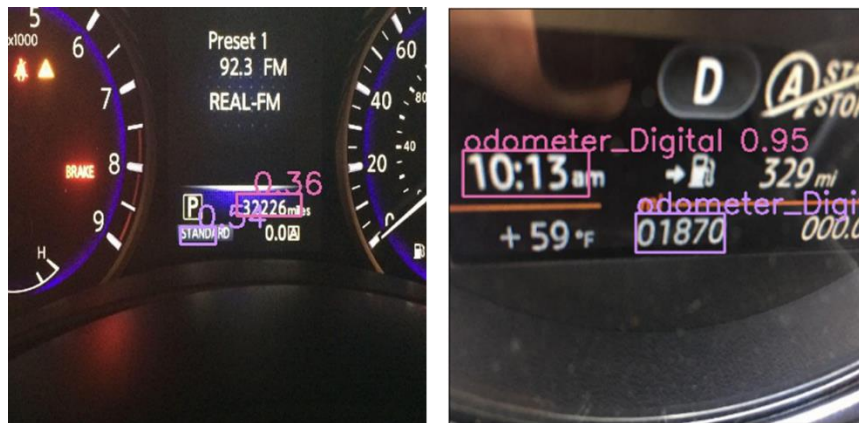
Figure 10. Two examples of false positive detections for the odometer detection model. The numeric value above each box shows confidence level in the detection. In the first example, the model was more confident in the word "standard" than the actual odometer, and in the second example the model detected two odometers.
