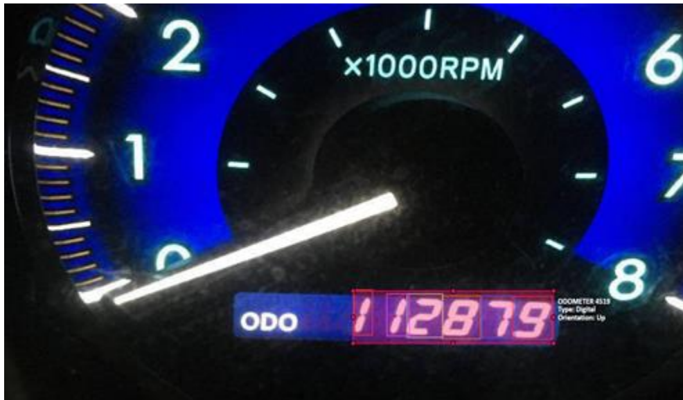
Figure 3. Example of the odometer and digit labeling in CVAT. Bounding boxes around the odometer region and individual digits were annotated along with additional metadata about the odometer such as type and orientation.
