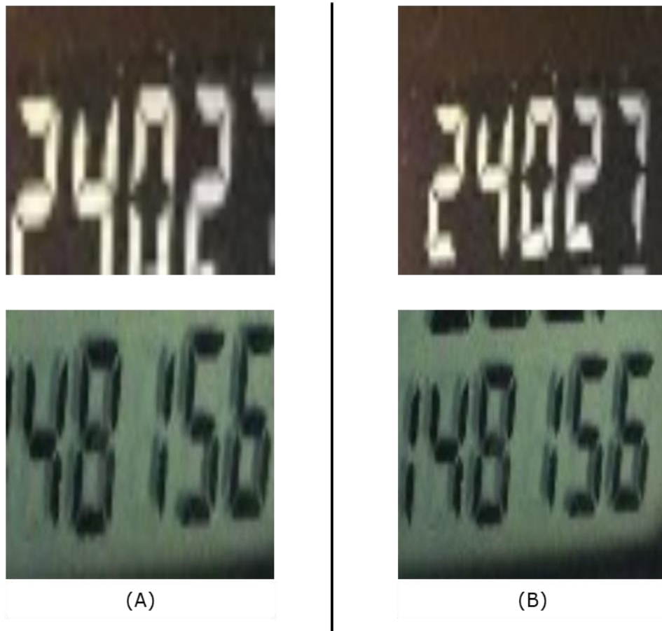
Figure 6. (A) Sample odometer crops based on bounding box output of the odometer detection model. The model tended to produce a tight margin around the odometer region which resulted in some digit getting trimmed. (B) We padded a few pixels along both row and column dimensions to ensure that all digits were accounted for.
