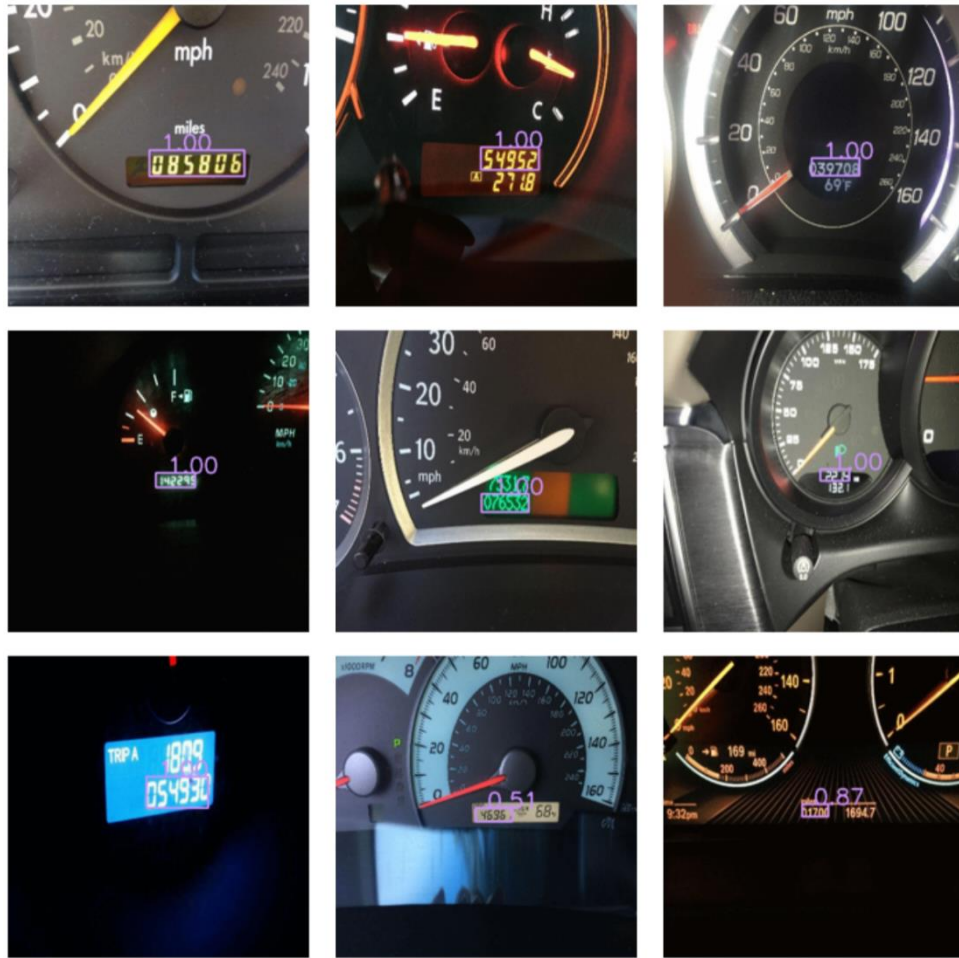
Figure 9. Example of a true positive detections for the odometer detection model. The numeric value above each box shows confidence level in the detection.
