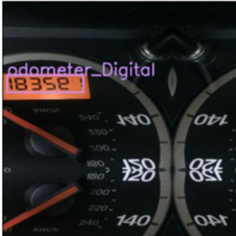
Figure 4. Example of augmenting a photo using pixel mirroring to make the odometer smaller. A large portion of the image is “fake”.
